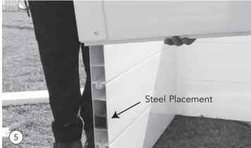
On a clean flat surface, assemble the well sections by sliding the sidewall onto the front wall as shown. Note that the inside of the front wall has a decal at the bottom and with units over 48" wide there are screws stabilzing the assembly on the back of the panel.
