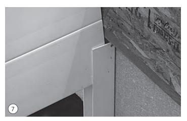
Carefully transfer the assembled well section to the mounting channel and slide it into the top, as shown.
